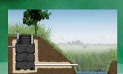
The treated water is discharged either underground (infiltration) or into water courses, depending on the ground type\*
