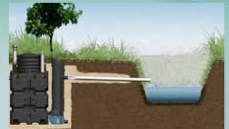
The treated water can be discharged by pump if required.
